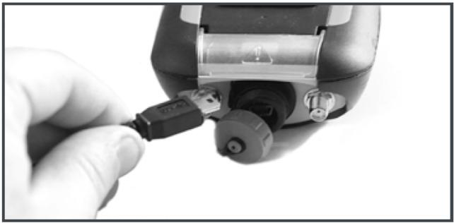
The estimated charging time to fully charge the device is 7 to 8 hours from completely discharged. The device can be used whilst charging, however, the charging cycle will complete more quickly if the device is deactivated. The device can be used with a partially charged battery.
