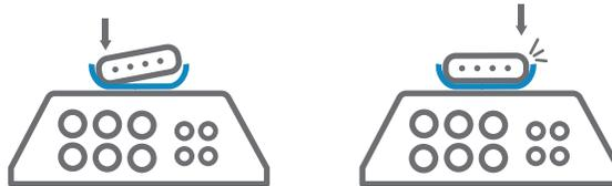
To remove the RockAIR from the mounting clip, move the top of the right side of the clip away from the RockAIR and lift the RockAIR clear.
