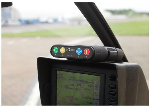
If you are unable to position the RockAIR anywhere with such a view, you should consider installing an external antenna or antennae. This is typically a dual mode GPS/Iridium antenna and a separate cellular antenna. This requires notification at time of purchase, or a return to your distributor for an approved modification.
